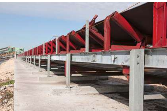
Multiple reclaim feeder units can feed a single conveyor allowing for material blending and increased tonnage.
