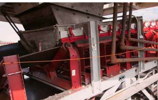
Working in combination, the Joy reclaim feeder, properly designed discharge chute and properly designed belt conveyor system work together as one unit.
