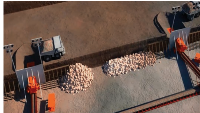
Joy feeder-breakers and sizers are utilized to process material in the pit.
