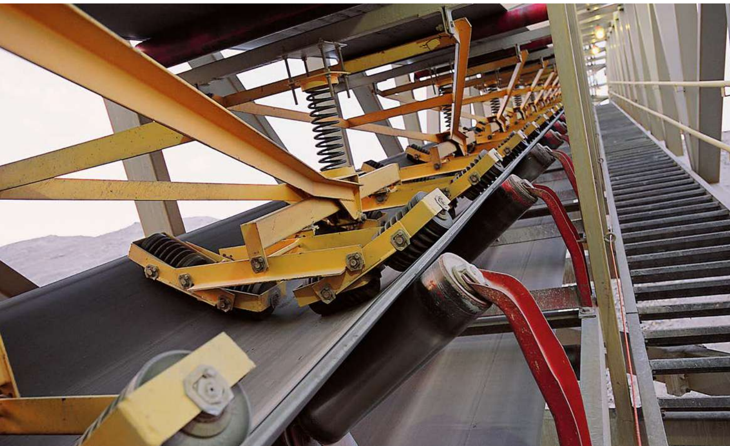
One of the secrets to the high performance capabilities of the HAC system technology is its use of pressing components.
