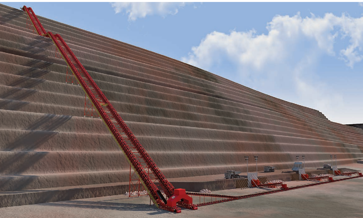
HAC systems elevate material from the pit on to overland conveyors for processing. A HAC system can convey material at very steep angles, high lifts and capacities over 8,000 MTPH, saving up to 50% in material handling costs.
