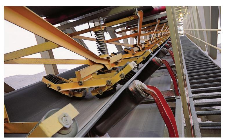
One of the secrets to the high performance capabilities of the HAC system technology is its use of pressing mechanisms.
